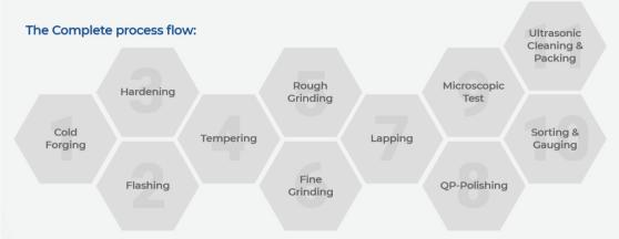
The balls are manufactured in less than 20.00 MM Dia in AISI-410, AISI-420, AISI-440C, AISI-52100, AISI-304, AISI-316 and Carbon Steel Grades
